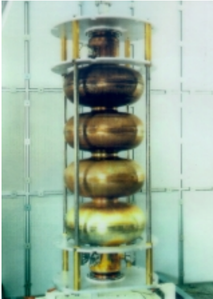
Figure 3. A 4 cell Niobium coated cavity in the clean room.
