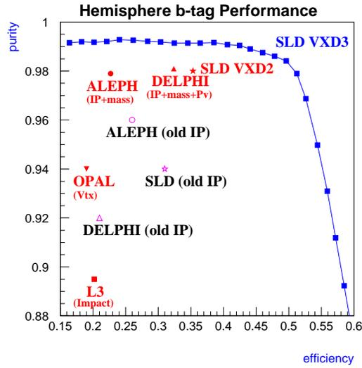
Figure 17: B-tag performances of the various experiments.
